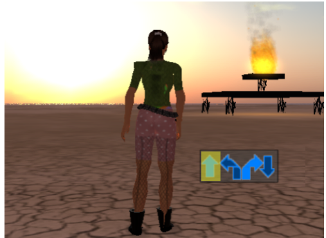
Figure 1: Hold-and-release scanning implemented in Second Life to navigate an avatar using a single switch. FORWARD and TURN RIGHT inputs are both selected and CANCEL FORWARD is highlighted.
