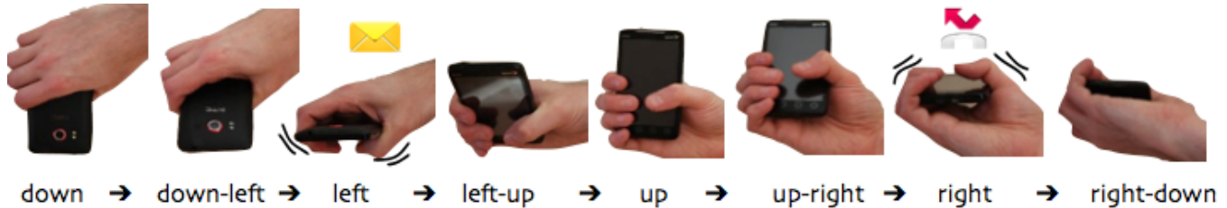
Figure 1: The user scans through eight different orientations of their mobile device where a specific target orientation is indicated using a vibrotactile cue. Different target orientations correspond to different types of information that the user can access in an ear and eye free manner. An example application of this technique indicates the status of a mobile device where LEFT indicates a new email and RIGHT a missed call.
