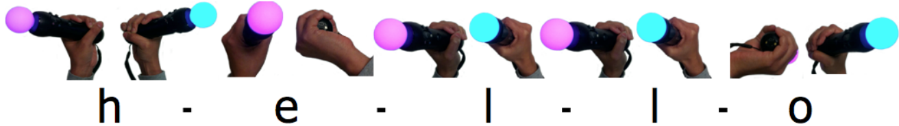
Figure 1: Combinations of different hand orientations define manual signs that correspond to different letters of an alphabet. For input, hand orientations are measured using low-cost mobile devices with integrated accelerometers, for output, users scan through a set of available orientations where a particular target orientation is indicated using vibrotactile feedback
